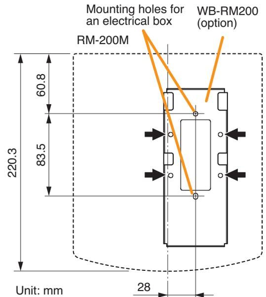
Use 4 mounting holes indicated by arrows to secure the WB-RM200 to the wall
